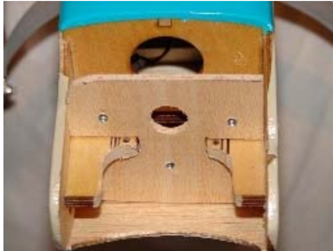
There are only 3 blind nuts to mount the motor, but that should be plenty!
