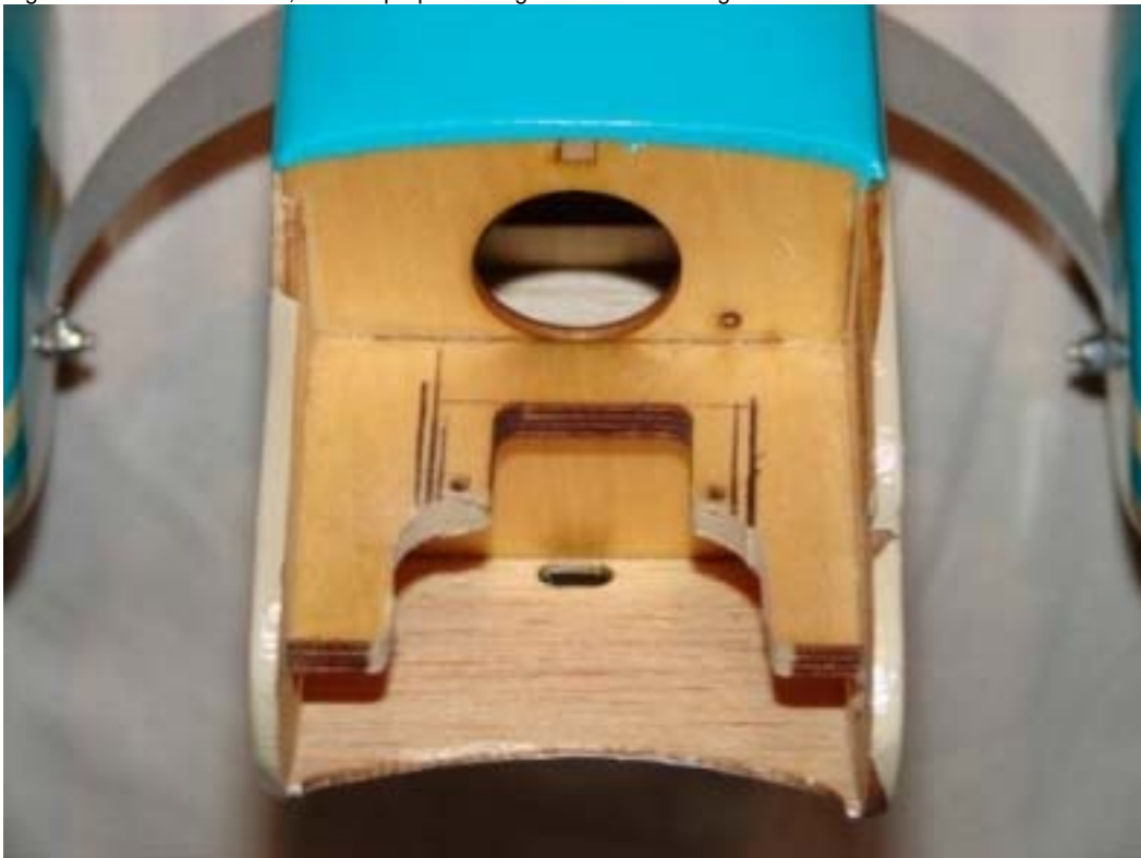
The trusty Dremel makes easy work of removing surplus ply from the engine mounting plate.
